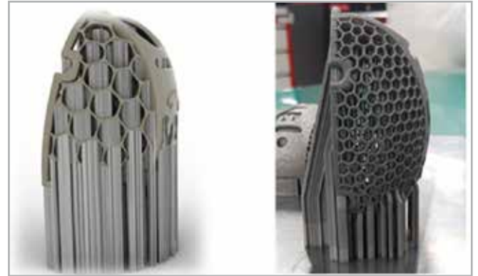
Fig. 8 - Supports in Alt 1 (left) and Alt 2 (right)
