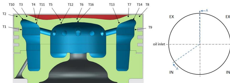
Figure 5: Temperature sensor locations inside piston
