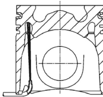
Figure 1: Piston jet cooling principle [1]
