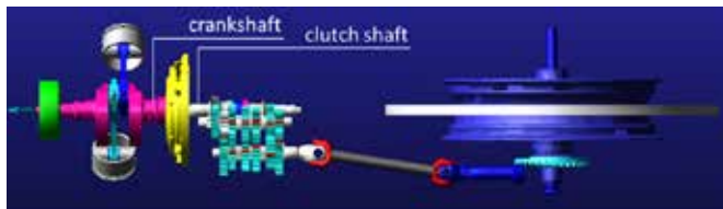
Figure 7 - Modelling remarks. Multibody analysis. Connection between the crankshaft and the clutch shaft. The crankshaft and the clutch shaft
