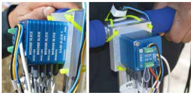
Fig. 8 - DAQ used for Strain Data Collection
