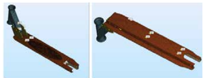
Fig. 5 - Virtual Strain Gauge Placement
