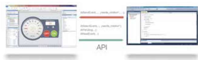
Fig. 4 - By allowing the connection of external tools that help define the application logic in parallel to the corresponding GUI parts, a connected GUI editor allows developers to develop and test in an agile manner.
