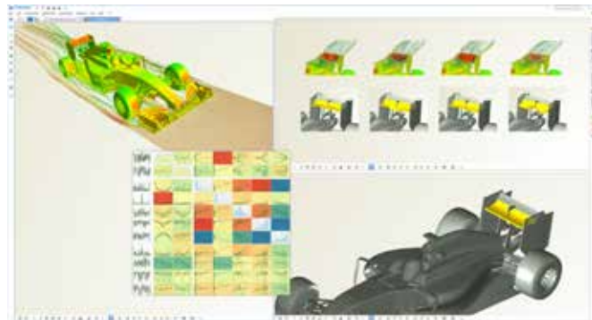
Fig. 1 - CAESES comes with specialized CAD, CFD automation, and an integrated optimization environment
