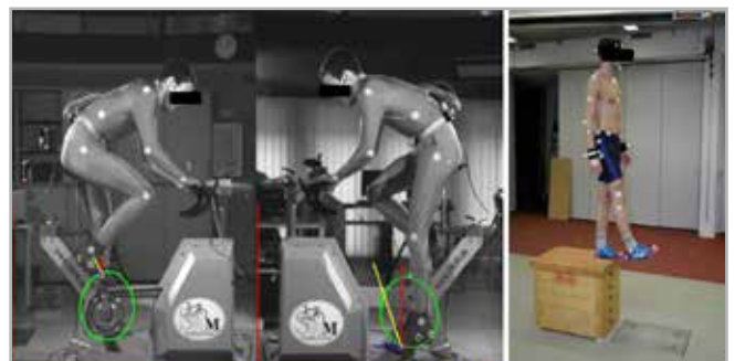
Fig. 8 - Two different motion capture systems: one based on visible light (left), one based on infrared cameras and reflective markers (right)
