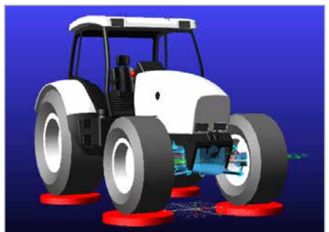
Fig. 3 - Example of an MSC Adams 4-poster model
