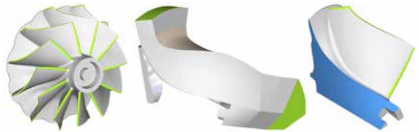
Fig. 3 - Parametric turbocharger turbine including parametric flow and structural domain for automated meshing
