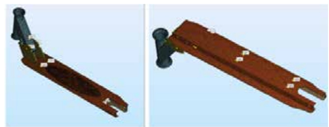
Fig. 5 - Virtual Strain Gauge Placement
