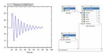
providing the user with the resulting pressure distribution all along the 2-km discretized pipe, at every time-step simulated.
