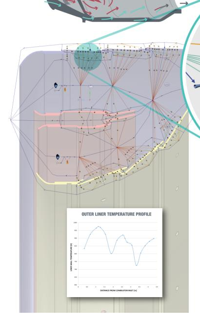
Preliminary combustor design requires that an extensive number of geometrical and operational conditions be evaluated and compared. Especially during this phase Flownex® is an essential tool for combustor design engineers as it accurately captures important parameters such as the mass flow rate distribution through air admission holes, associated pressure losses as well as liner wall temperatures.
